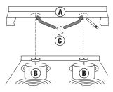
Use the enclosed prep pad (C) to clean the areas in range hood (A) where the magnet of each suppressor unit (B) will mount\*. Make sure area is completely dry & free of grease.
