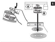
Carefully remove existing product (B) by grasping the unit by the mounting post and twist to disengage the magnet.
