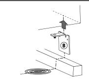
Slide wall bracket up to touch bottom of microwave or cabinet.
