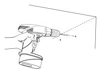
Drill 1/8" pilot holes in the marked locations. If wood stud is present behind drywall, proceed to Step 7.
