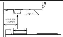
The center of the rear canister must be over the rear burner. If not, go to www.STFS.com to order an extension bracket kit.
