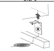
Slide wall bracket up to touch bottom of microwave or cabinet.
