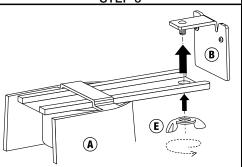
Secure main unit [A] to wall bracket [B] with wing nut [E]. Do not overtighten. Installation is complete.
