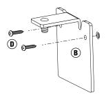
Align bracket [B] and attach with screws [D] (or use hardware suitable for your backsplash material).
