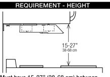
Must have 15-27" (38-68 cm) between surface of stove top and mounting point under microwave hood.
