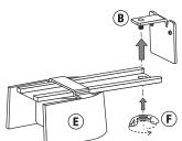
Secure main unit (E) to wall bracket (B) with wing nut (F).
