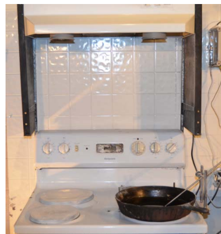
Figure 3. Stovetop Firestop® Installed Prior to a Fire Test.
