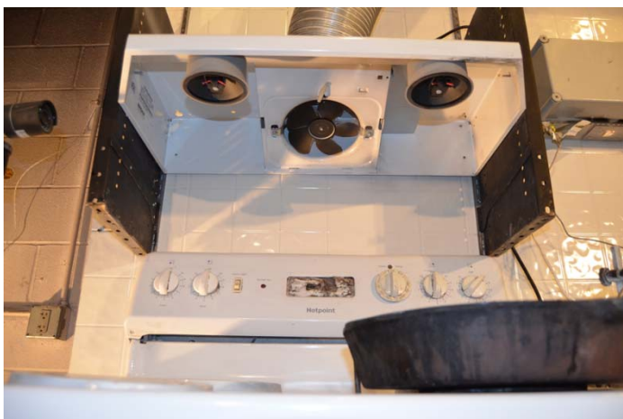
Figure 3. Stovetop Firestop® Installed Prior to a Fire Test.
