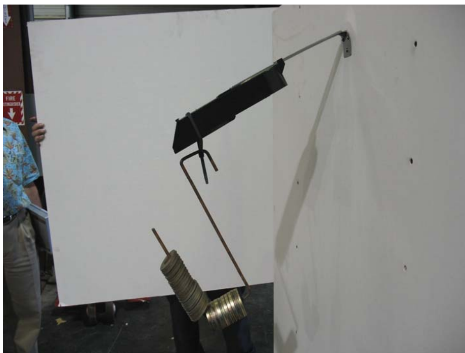
Photograph No. 5 Wall-Mount, Full-Weight Test
