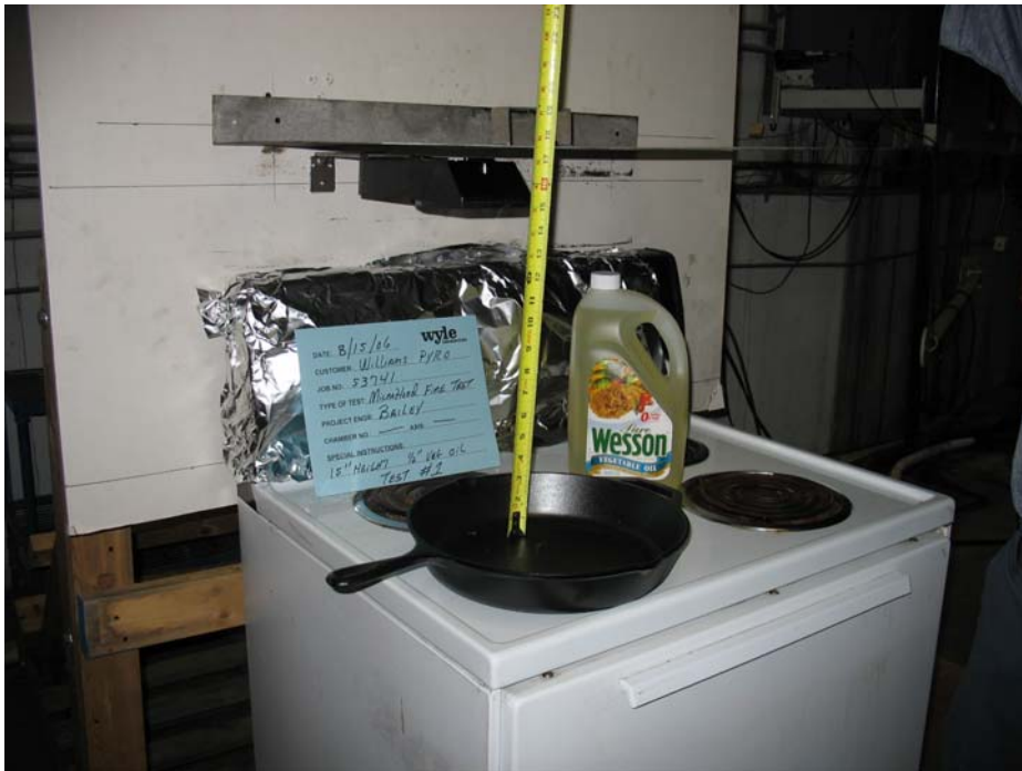
Photograph No. 2 Test Setup, 15-Inch Installation Test
