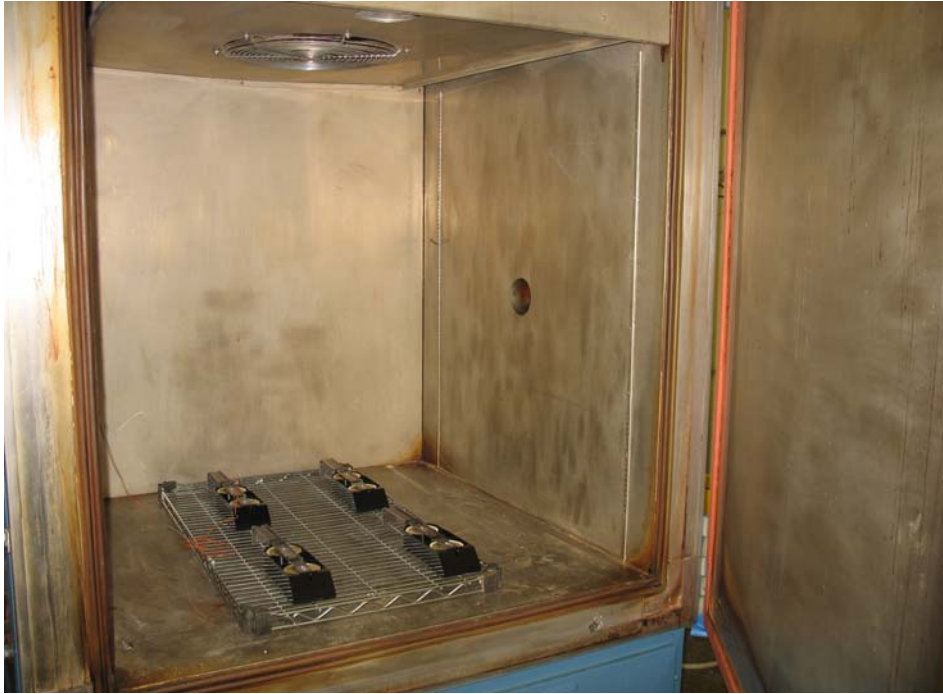
Photograph No. 3 Temperature Conditioning Setup
