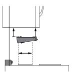
Raise the unit to the bottom of the microwave or ventilation hood without attaching the magnet arms.
