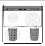
Position the units on the stove magnets up, where the units front fuse is facing toward the front of the stove.
