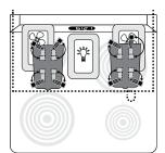
Take note of where the magnets could come in contact with fan vents, lights, or other obstructions.
