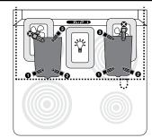
Make sure at least three (3) of the four magnets are firmly secured to the bottom of the microwave.
