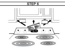
Place the enclosed decal under or near the microwave where it can be seen.
