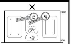
VENTS: Canisters should not be mounted over any vents, if possible. The ClickBar and magnets may do so, but only if it permits the device to meet the three (3) magnet minimum requirement. Some metallic parts under the microwave may not hold a magnet.
