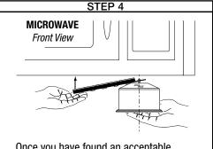
Once you have found an acceptable location, lift the ClickBar upwards. Confirm that three (3) of the five (5) magnets are securely fastened.
