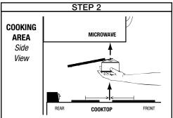
Raise canisters from underneath to the spot directly above under microwave without attaching the ClickBar.
