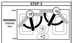
Use one hand to hold the canister in its final position, while using the other hand to swivel the ClickBar to the optimal mounting position (see precheck section).
