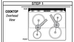
Position the canisters on the stove where the canisters sit at the midpoint between the center of the front and back burners on each side. The ClickBar need only be able to be raised without obstructions.
