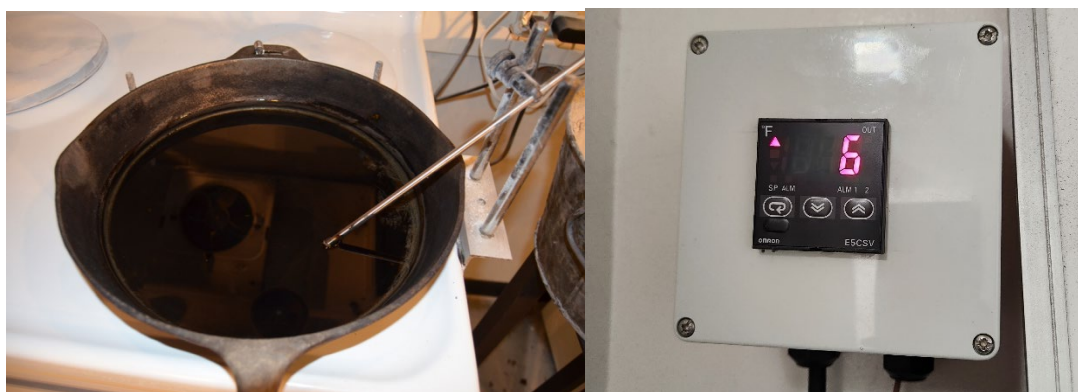
Figure 5. Oil Temperature Measurement (Left: Thermocouple Probe, Right: Temperature Display).
