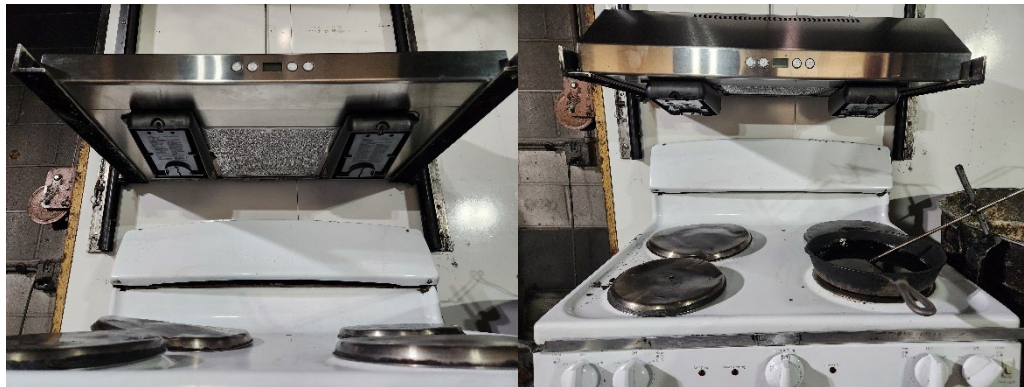
Figure 3. Stovetop Firestop® LowPro® Installed prior to a Fire Test.
